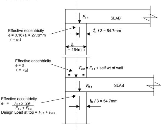
Alternatively, for walls with a minimum compressive stress above the joint of 0.25MPa or with reinforcement that can resist the design moment, a rigid frame analysis may be used.
