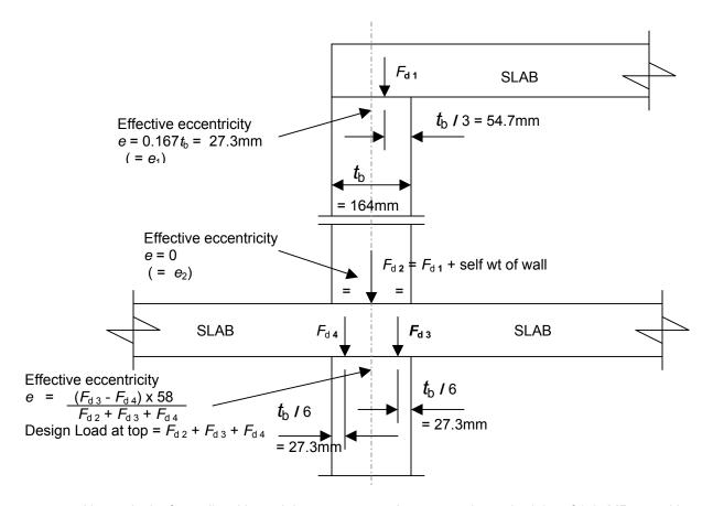
Alternatively, for walls with a minimum compressive stress above the joint of 0.25MPa or with reinforcement that can resist the design moment, a rigid frame analysis may be used.
