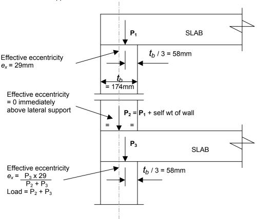
Note: in the above diagram  $t_b$  is the equivalent bedded thickness of the wall = 174mm
